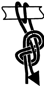
Fig of 8 as a Hitch
