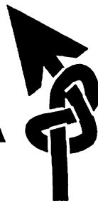
Fig of 8 as a Hitch
